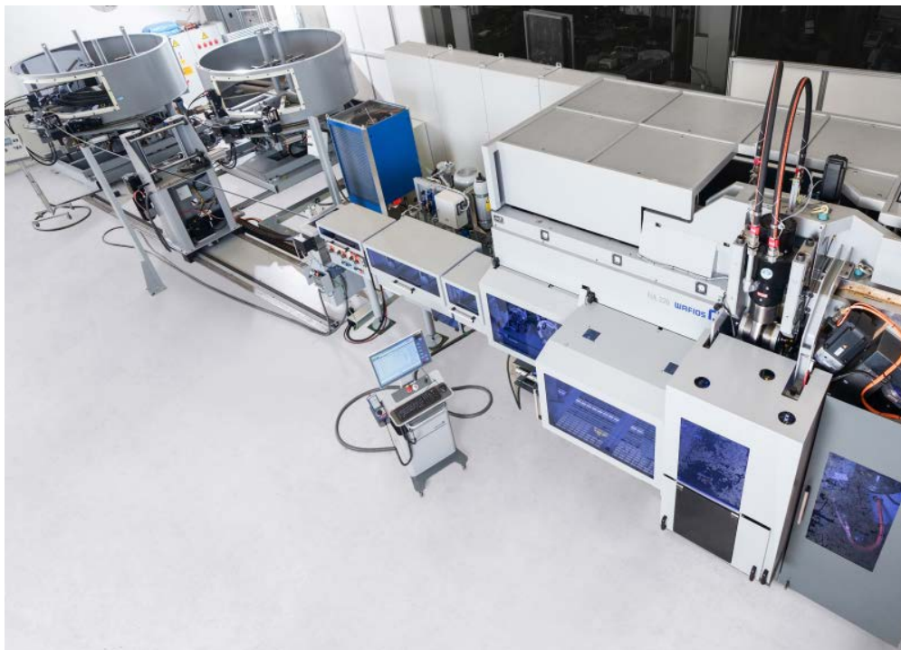
Fig. 2 FUL 226 with dual-coil pay-off unit
