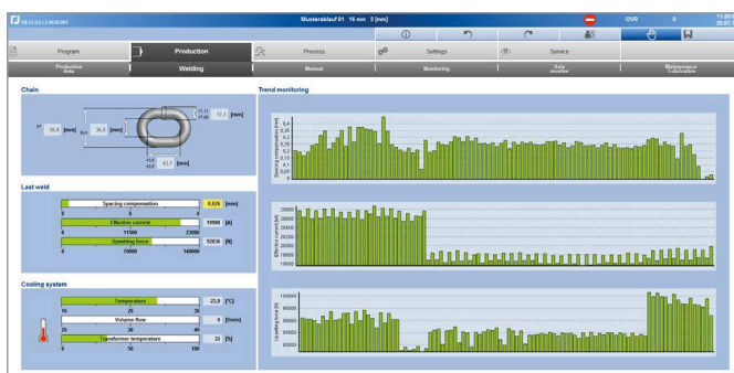
▲ Monitoring of the welding process
